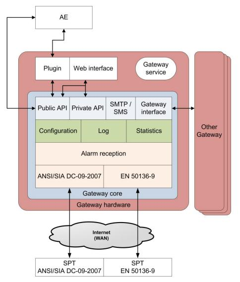
The IP-RCT work, in reference to EN-50136-3, in pass-through mode. This operating mode means that no signals are stored until acknowledged by an annunciation equipment (AE).
